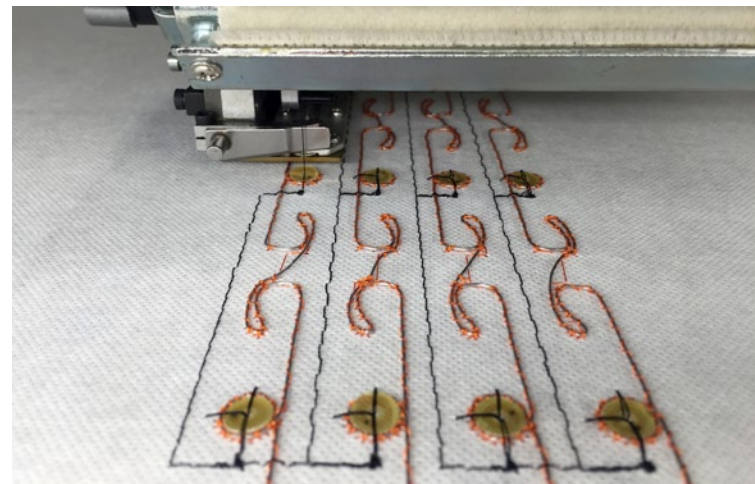
Fig 17- Functional Sequin for automated Placement of RFIDs
